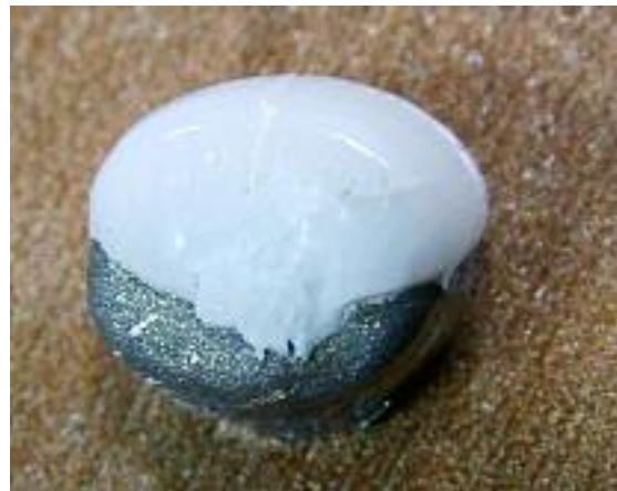
Figure 3. Mixed failure, loss of one second of the veneer material of lower first molar (Original magnification X10)
