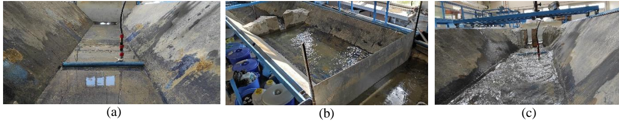
Figure 1. Experimental Setup (a) no weir (b) V-weir (c) E-weir
