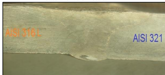
Fig. 5. Macroscopic images of the weld bead, of dissimilar welding of AISI 316L and 321 type metal couples –base and weld metals.
