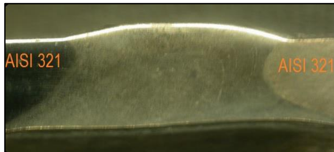
Fig. 3. Macroscopic image of the weld bead, of similar welding of AISI 321 type metal couples – base and weld metals- .
