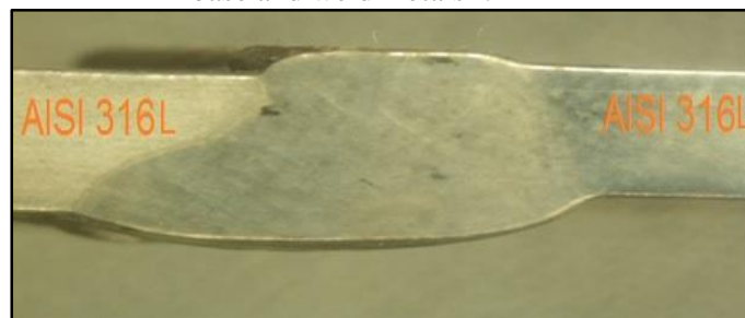
Fig. 4. Macroscopic image of the weld bead, of similar welding of AISI 316L type metal couples – base and weld metals.
