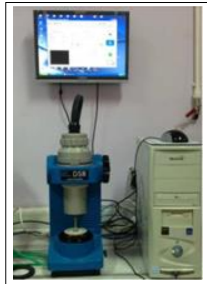
Figure 3. The dynamic shear rheometer test device.
