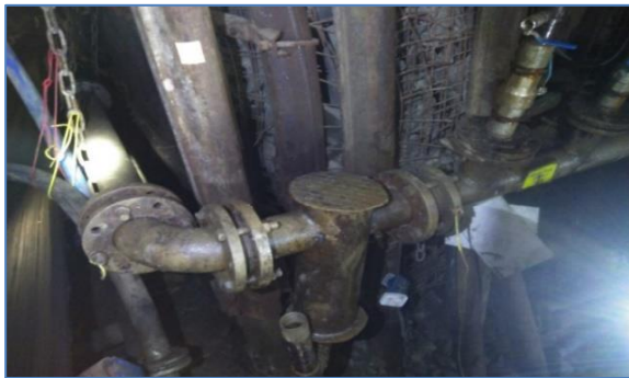
Şekil 10. Metan drenaj boru şebekesinden su tahliye sistemi. Figure 10. Water evacuation system from methane drainage pipe network.
