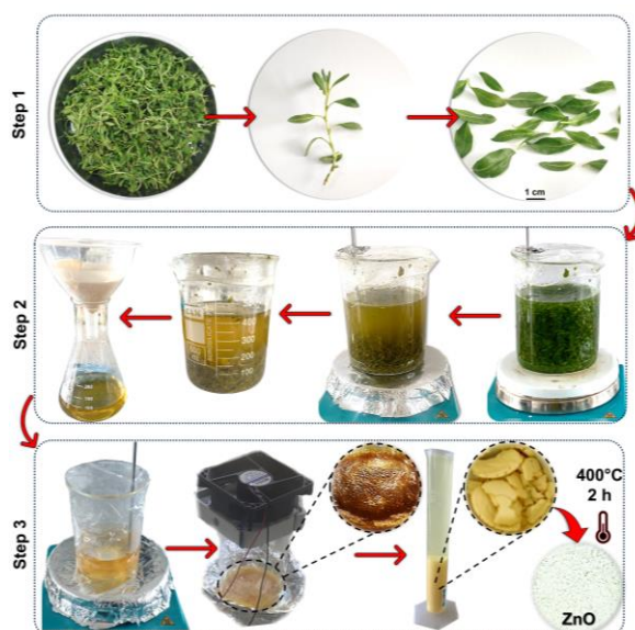
Figure 1. Detailed processing steps for the green synthesis of zinc oxide particles
