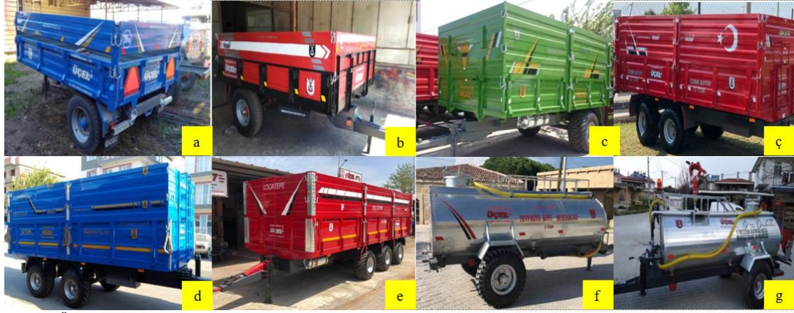
Figure 1. Agricultural trailers and liquid tankers manufactured by Üçel 17 Ltd (a: 2.5 tons agricultural car b: 3.5 tons agricultural trailer c: 5 tons agricultural trailer ç: 12 tons agricultural trailer d: 18 tons agricultural trailer e: 24 tons agricultural trailer, f: 3 ton water tanker g: 5 ton fire extinguishing tanker)
