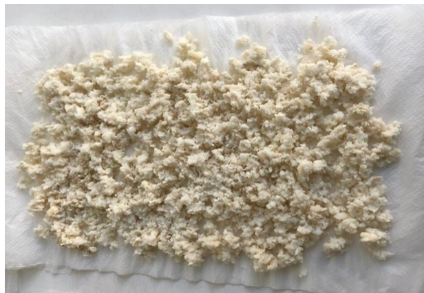
Figure 1. Paper pulp obtained with \text{NaClO}_2 method
