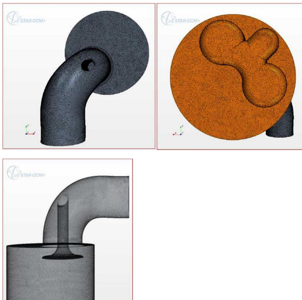
Fig.5 Element Distribution of The Continuum.
