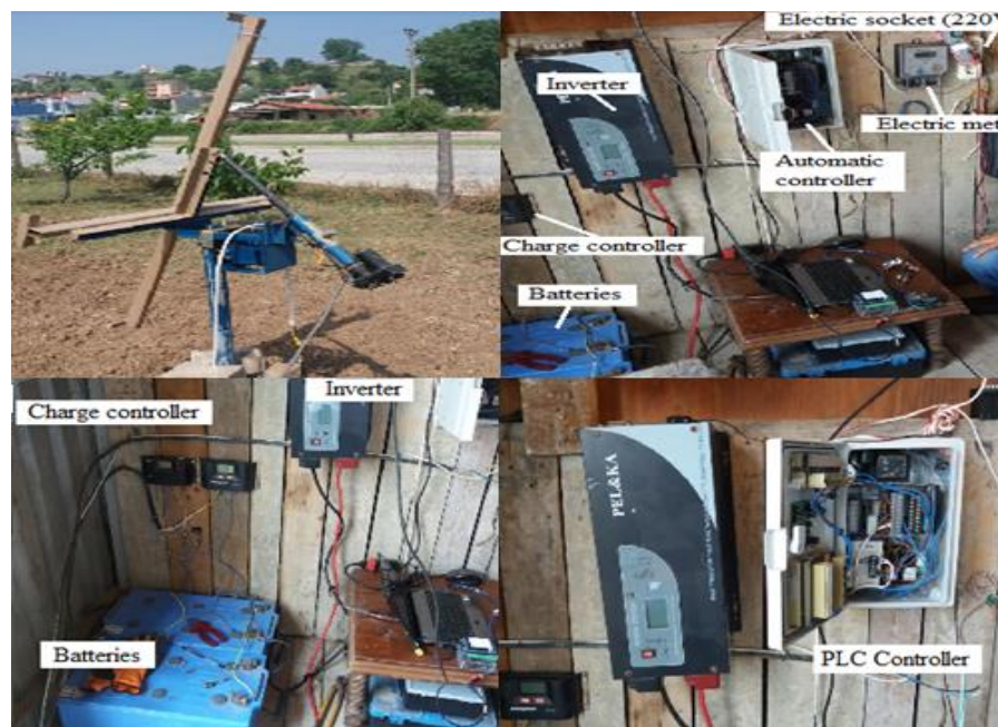
Figure 6. All apparatus (inverter, batteries, electric meter, data logger and etc.) used in the experiment
