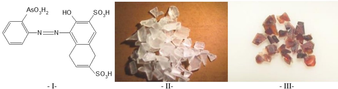
Figure 2. Open chemical structure of Thorin (I) and pictures of Unmodified PVA (II) and Thorin immobilized PVA (III)
