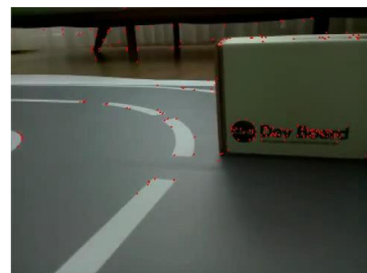
Figure 13. Corner detection on the image with FAST algorithm.
