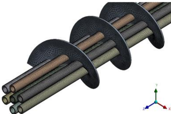
Figure 3. Isometric view of mesh structure of the heat exchanger (Case-III)
