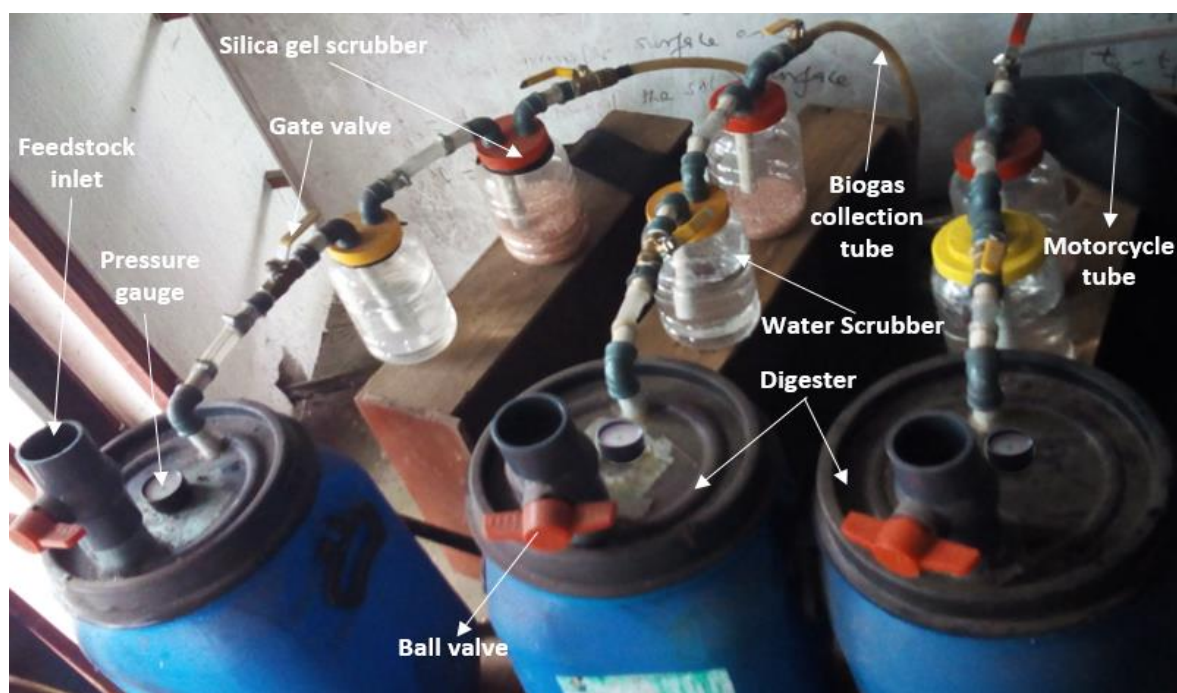
Figure 2. Experimental Setup for Anaerobic Digestion of Food Waste
