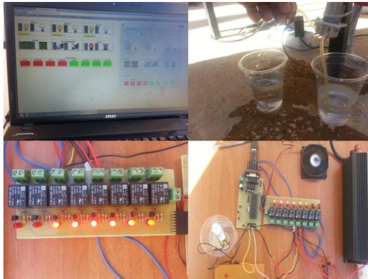
Fig.10. Observation of led and loads with all active output
