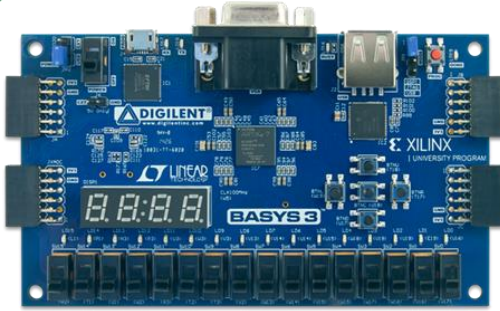
Fig. 4 BASYS3 FPGA training card
