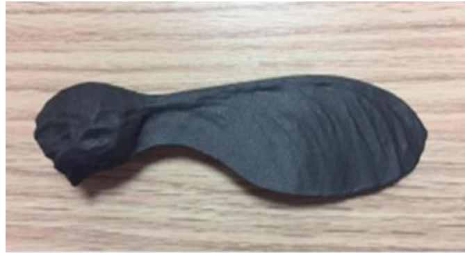
Figure 4. Prototype aerodynamic bionic wing manufactured with 3D MJF Technology
