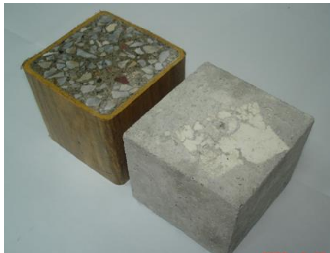
Figure 1. Concrete and hybrid compression samples
