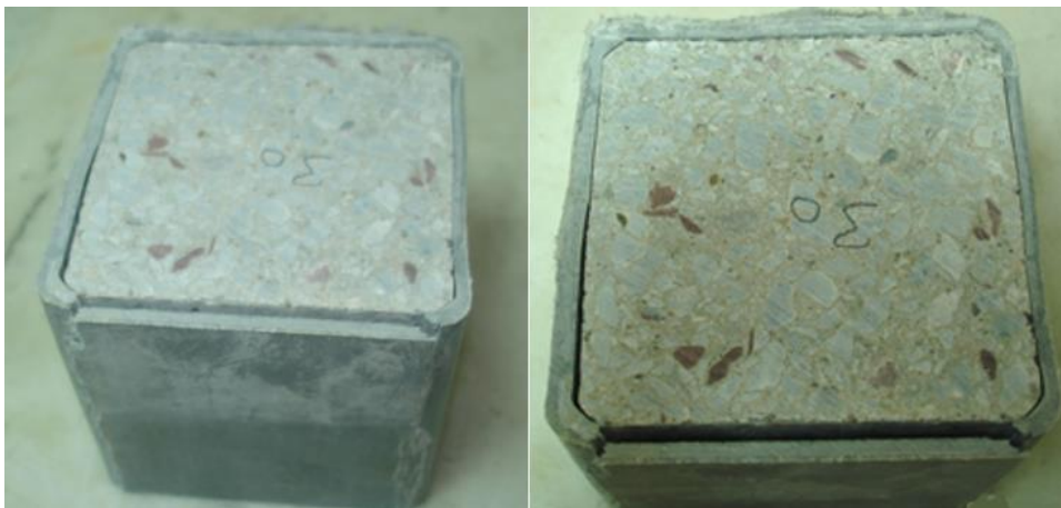
Figure 11. Failure modes of hybrid samples
