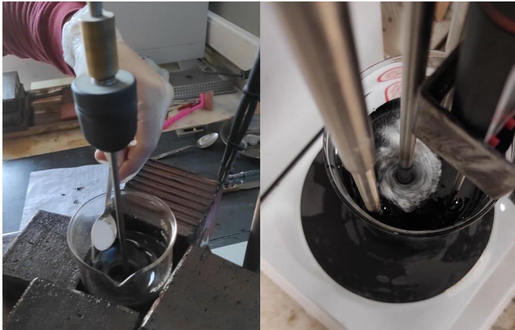
Figure 6. Production of PVC Waste-Modified Bituminous Material
