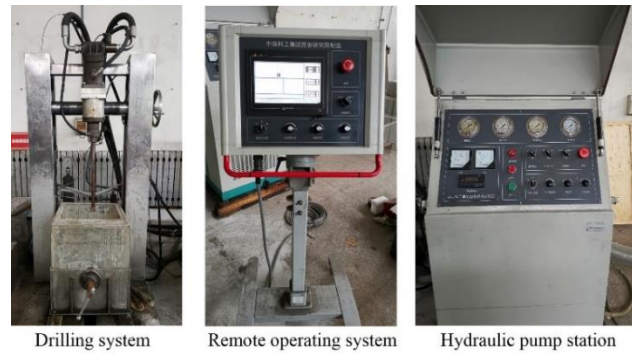
Figure 13. Main components of micro-drilling test device
