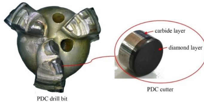
Figure 1. PDC drill bit wear photo
