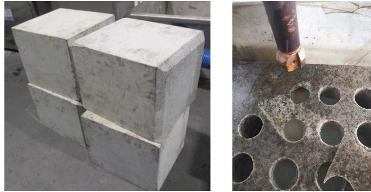
Figure 15. (a) Rock sample b) the photo after drilling
