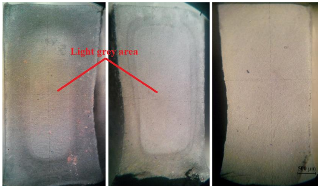
Figure 4. Cross-sectional view of samples after sintering (a: 1200 °C 120 min., b: 1200 °C 240 min., c: 1250 °C 240 min.)
