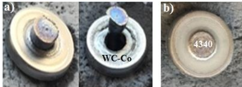
Figure 2. Sintered samples (a: 1350 °C, b: 1300 °C)
