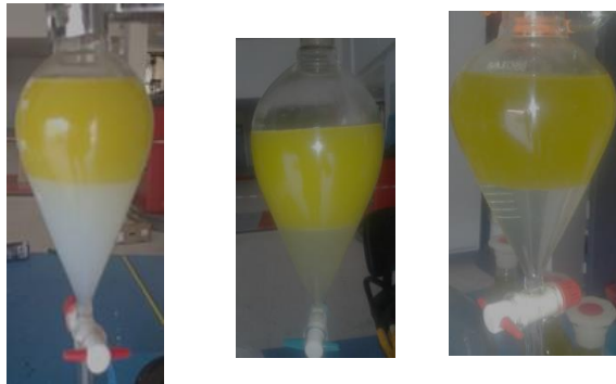
a) First washing b) Second washing c) Third washing Figure 1. The washing process of biodiesel
