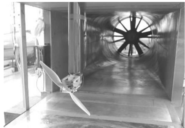
Figure 4. Wind Tunnel Used for Propeller Testing [6]
