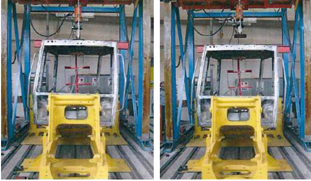
Fig. 16. Vertical loading (before &amp; after test).
