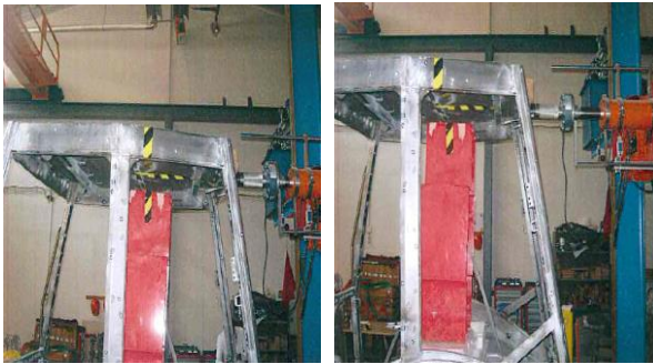
Fig. 17. Longitudinal loading (before &amp; after test).
