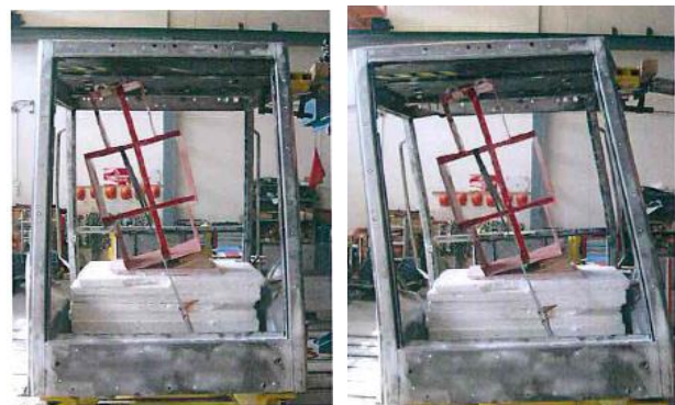
Fig. 15. Lateral loading (before &amp; after test).
