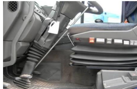
Fig. 5. Brake pedal apparatus assembly [5]
