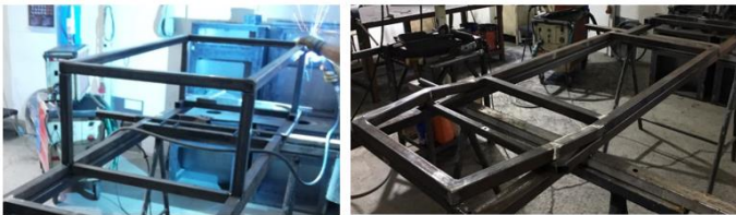
Fig. 20. a) Chassis manufacturing b) Welded chassis
