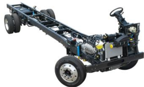
Fig. 3. Ladder type chassis [35]
