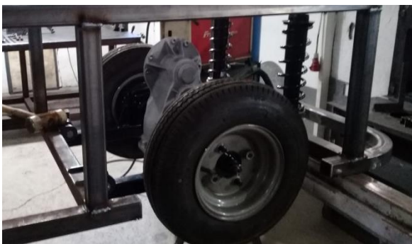
Fig. 21. Suspension and wheel system installation
