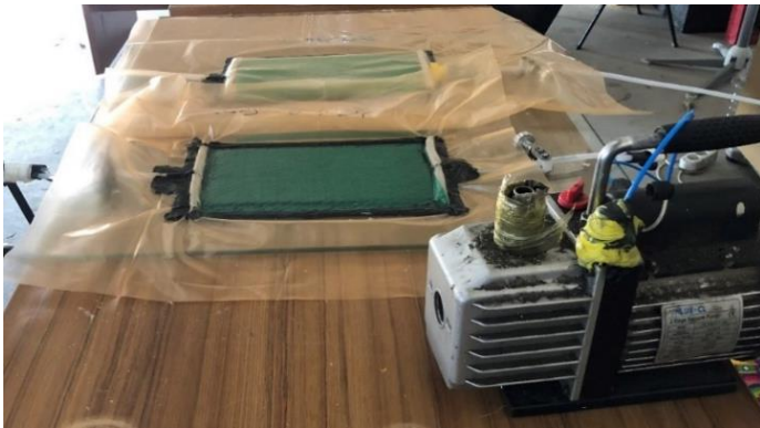
Fig. 3. Vacuum assisted resin transfer method
