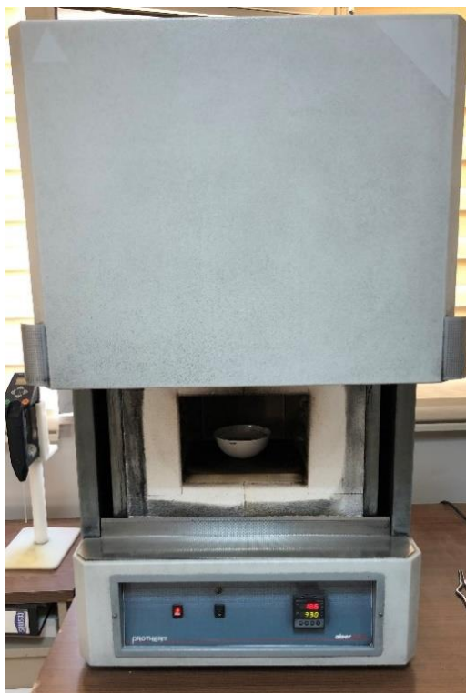
Fig. 6. Composite samples in a porcelain crucible in an electric ash furnace
