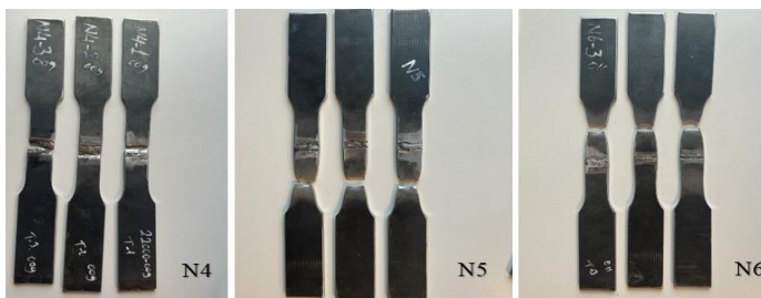
Fig.6 SMAW welded samples' photographs after tensile test
