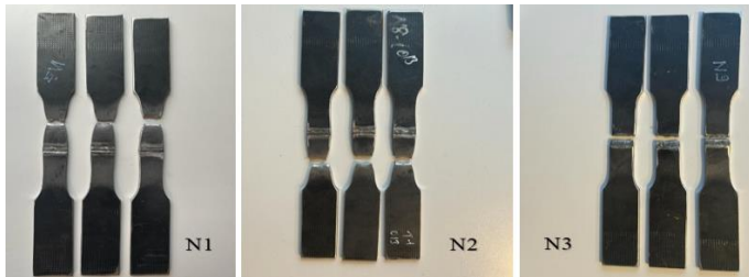
Fig.5 MAG welded samples' photographs after tensile test
