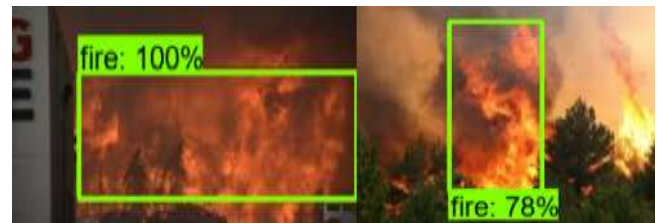
Figure 2. SSD fire detection model on test images.
