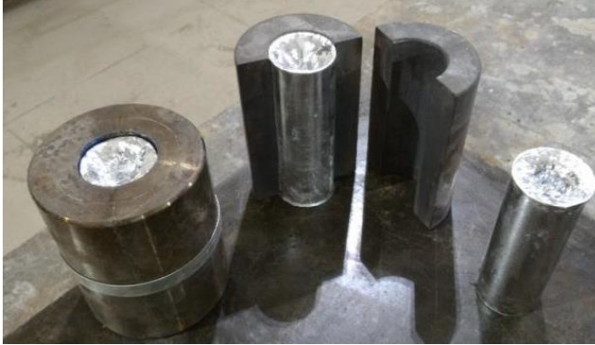
Fig. 1. Pre-samples and steel molds
