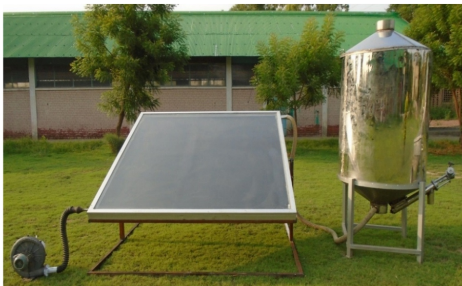
Figure 3. Actual view of solar sustained batch type maize dryer.
