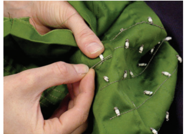
Figure 6. Conductive yarn with LEDs [14]
