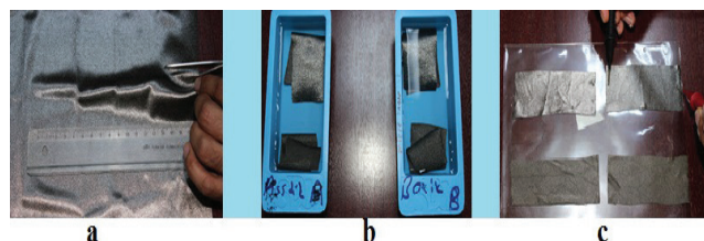
Figure 8. Preparing and measuring of the patterns (a: cutting of the patterns, b: putting the samples into solution, c: measuring the resistance of patterns)
