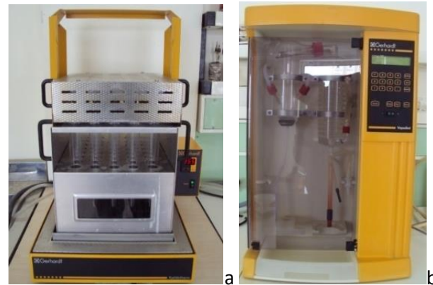
Figure 2. Kjeldahl digestion (a), Kjeldahl distillation and titration (b)
