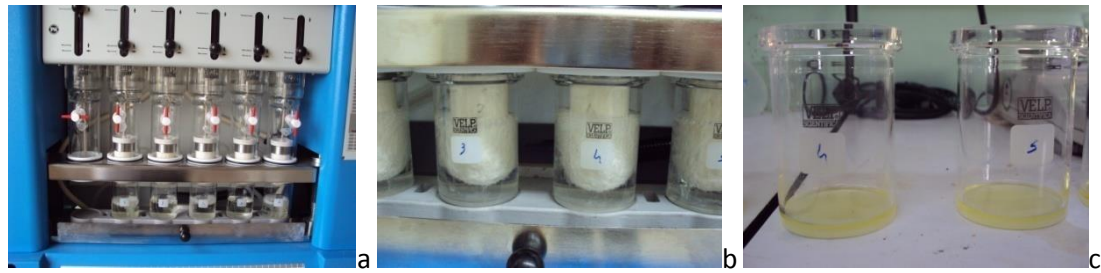
Figure 4. Soxhlet extraction (a), working of soxhlet extraction (b), fat extraction (c)
