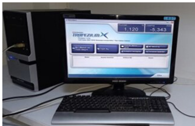
Figure 4. Trapezium X materials testing software compatible with Universal testing machine
