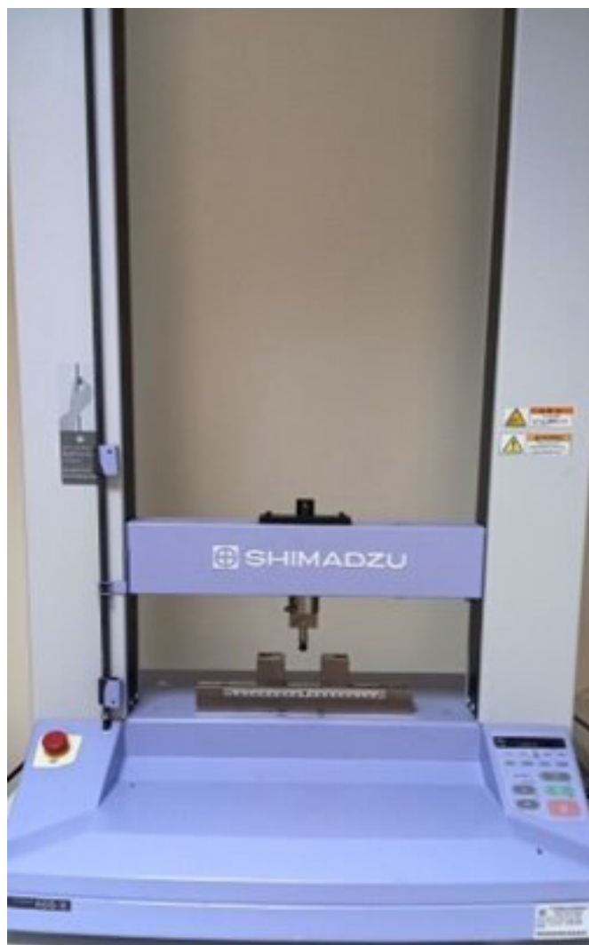
Figure 3. Universal test device used in the study
