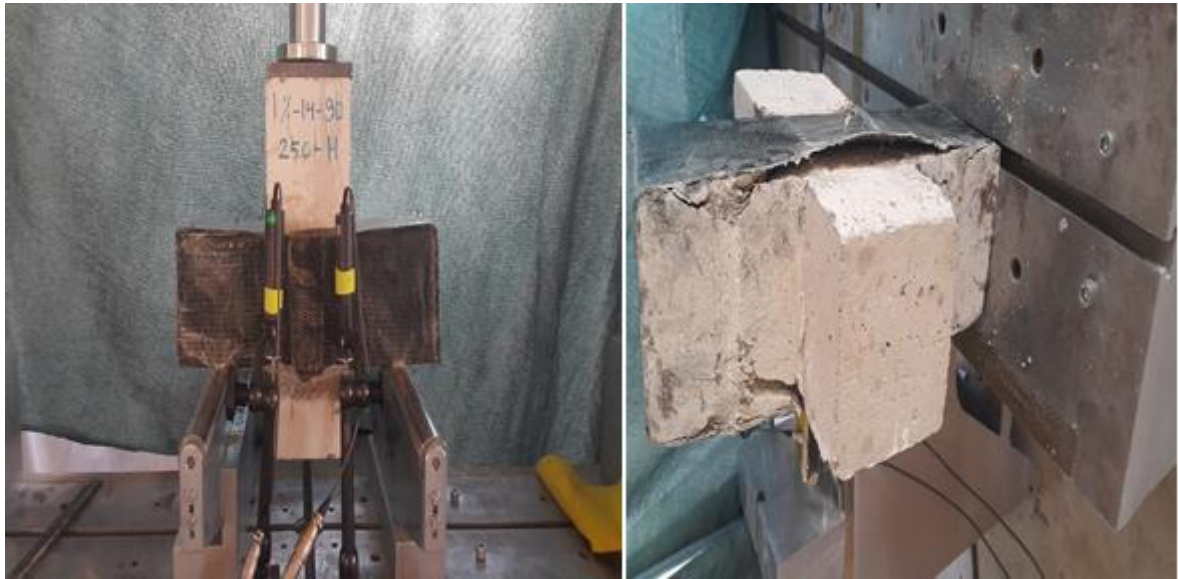
Figure 5. Specimen with De-bonding failure
