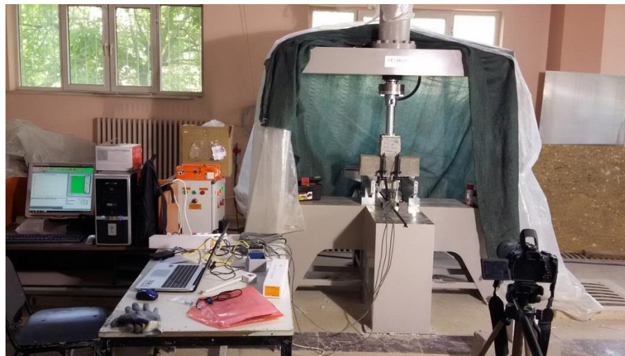
Figure 4. Corbel Specimen Setup
