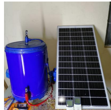
Figure 4. Experimental prototype of all systems: PVT collector.
