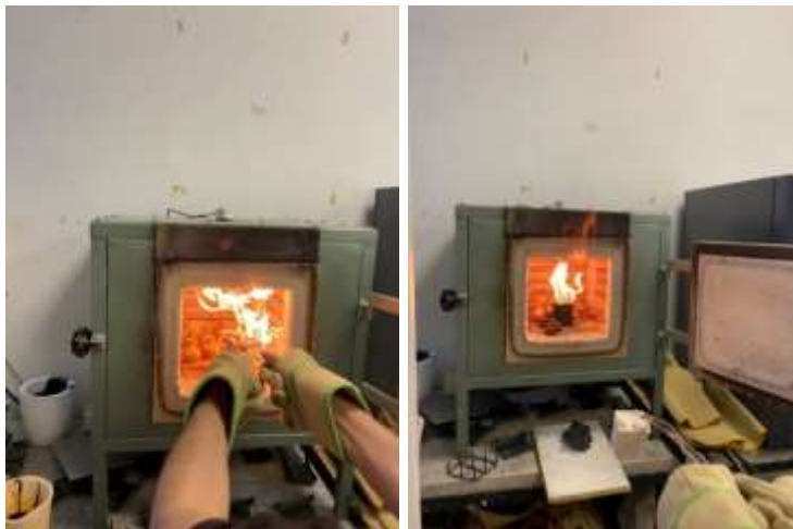
Figure 8. Placing the ceramic pots in the kiln.
