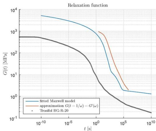
**Figure 6.** Fitted relaxation function of the interlayer Trosifol® Extra Strong for the reference temperature  $20^\circ\text{C}$  and comparison with previously tested Trosifol® BG-R-20.
