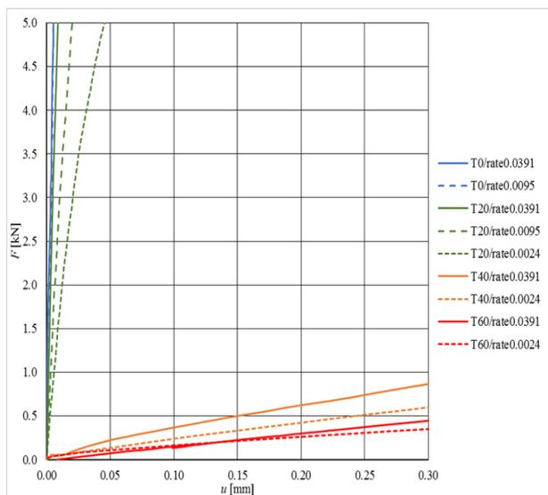
**Figure 7.** Force-displacement relationships determined experimentally by static loading with constant strain rate 0.0391; 0.0095 and 0.0024 s<sup>-1</sup> at the temperature of 0; 20; 40 and 60 °C
