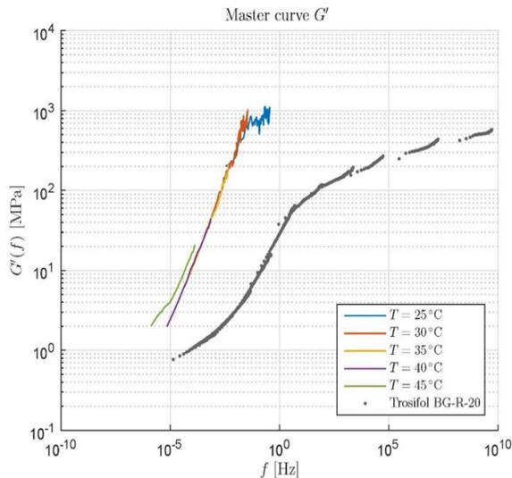
**Figure 5.** Constructed master curve of interlayer Trosifol® Extra Strong for the temperature  $20^\circ\text{C}$  and comparison with previously tested Trosifol® BG-R-20.
