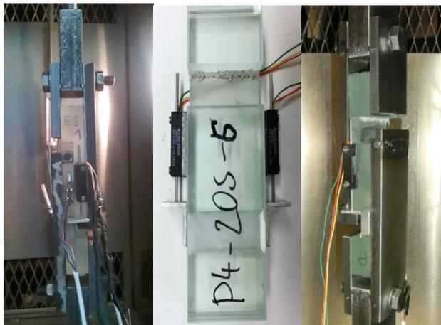
**Figure 3.** Test arrangement: a) arrangement in case of DMTA (testing specimen in climatic chamber), b) testing specimen of laminated glass with displacement transducers, c) arrangement in case of quasi-static test.
