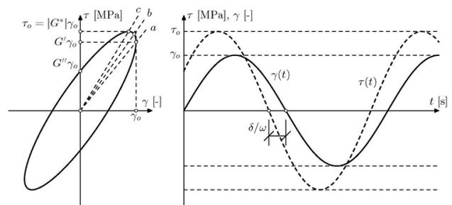
**Figure 1.** Cyclic loading of viscoelastic material: stress-strain diagram and phase-shift between engineering strain and stress functions in time
