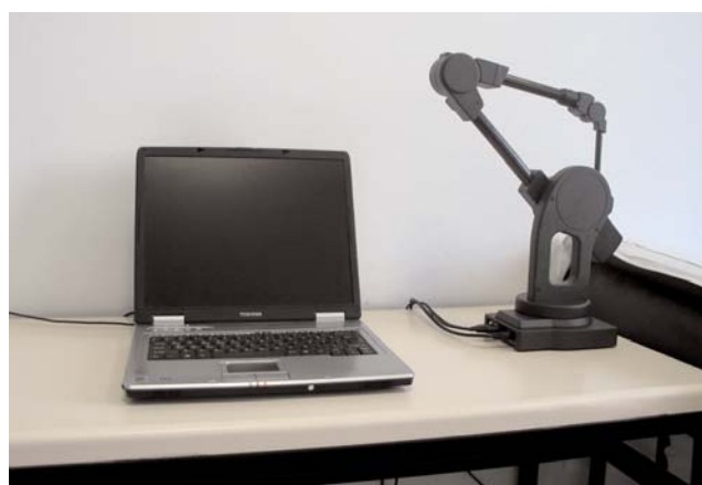
Figure 2. Microscribe digitizing system.
