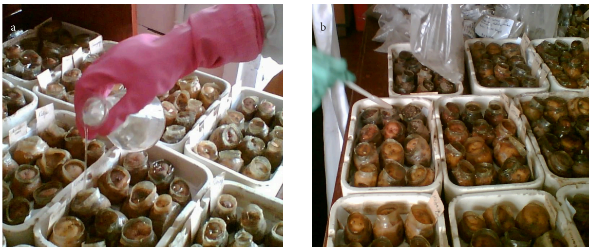
Figure 1. Experimental design showing the pathotype differentiation of Synchytrium endobioticum . a) Filling the eye fields encircled with vaseline + paraffin (1+1) with water, b) Addition of compost to the watered area
