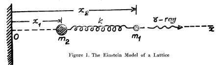
Einstein model of a lattice and it is an oscillator of single vibrational mode of frequency  $w=(k/\mu)^{1/2}$  where  $\mu$  is the reduced mass of the system.
