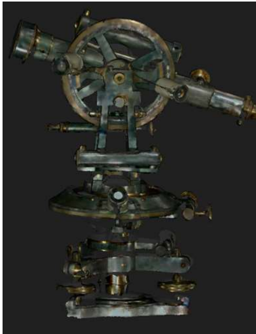
Figure 7. 3D scanning model of the theodolite.
