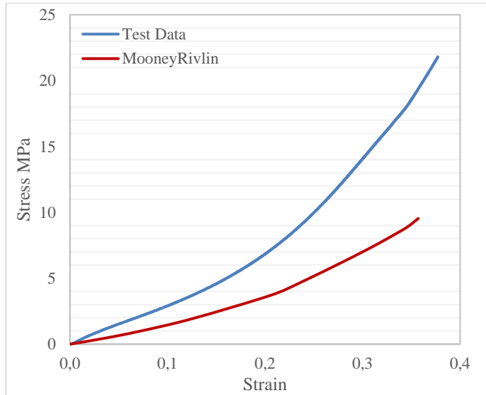
Figure 8 Stress-Strain curves for polynomial models
