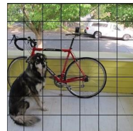
Figure 7. YOLOv4 Divide the Input into S X S Grid Cells (Joseph Redmon et al., 2016)
