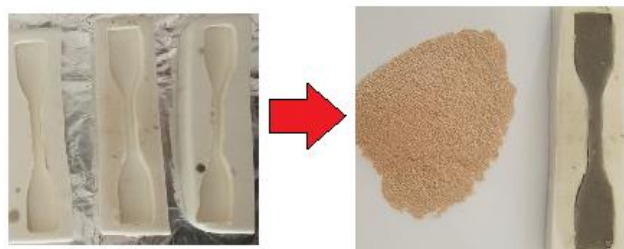
Figure 2. Polyester composite production scheme
