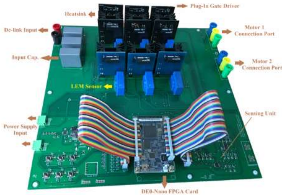
Figure 8. Annotated photography of the nine-switch converter prototype consisting of an FPGA evaluation board.
