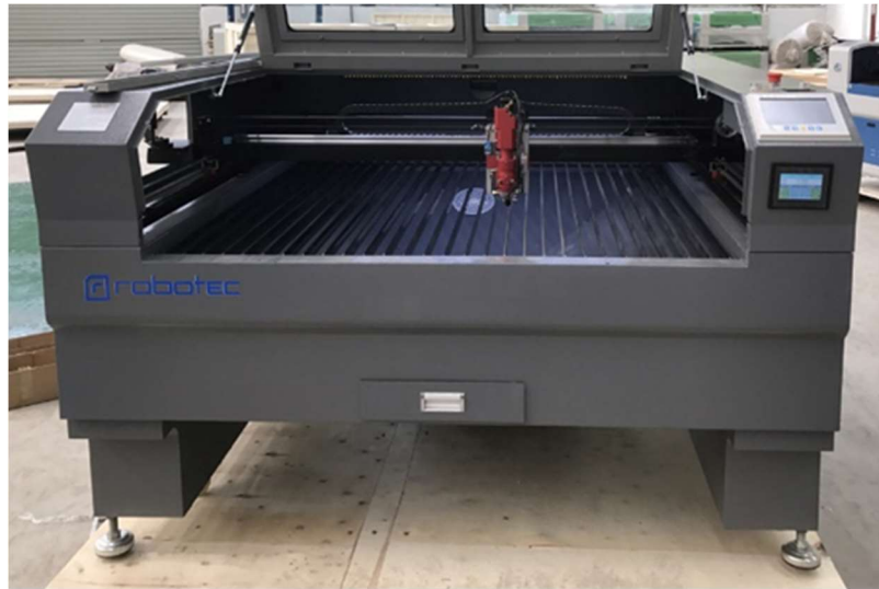
Fig 1. CO 2 laser cutting device used in the study
