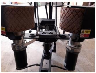
Figure 3. Ball thrower wheels and their motors
