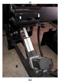
Figure 6. Horizontal-Vertical movement pistons and motors (a) Horizontal movement (b) Vertical movement
