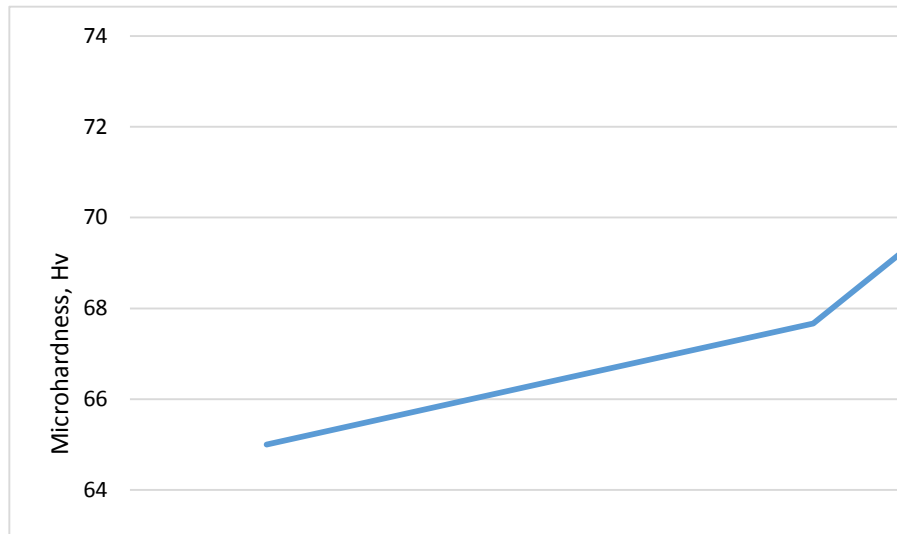
Figure 1. Microhardness change versus aging heat treatment
