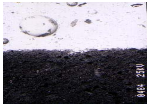
Fig.4 SEM mic.grph., Samp.7 Coloured glaze brick piece
